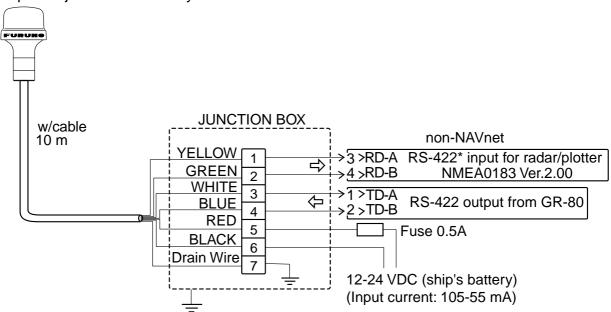
\*: RS-422 output can be received by current loop.
